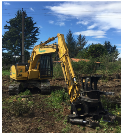
Tree shears provide controlled felling near power lines.
